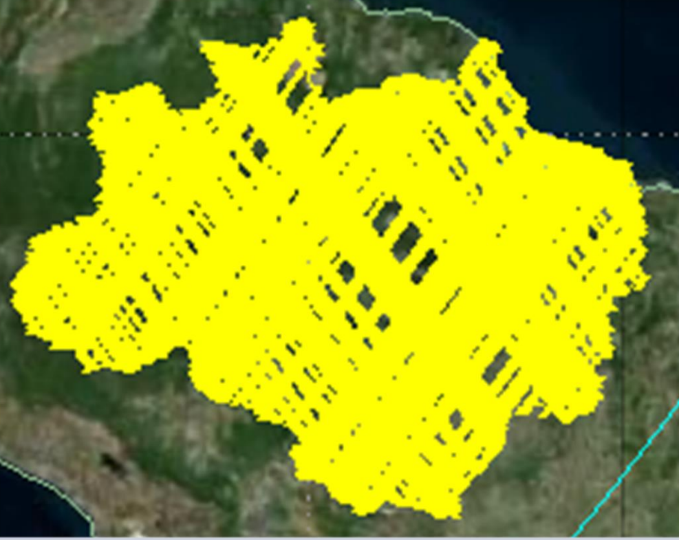
Figure 3. First scenario - Accesses between the CubeSat's payload and the Amazon rainforest (in yellow the areas that were scanned by the CubeSat).
